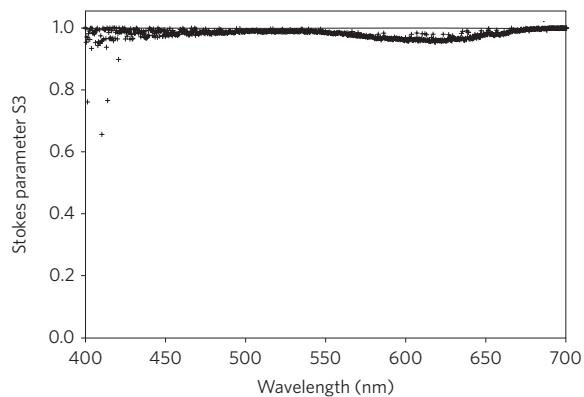
**Figure 2 | Achromatic conversion of linearly to circularly polarized light by the R8 cell.** Comparative experimental measurements (points) and calculated minimization (line) of the normalized Stokes parameter S3 for an ideal quarter-wave R8 retarder.
