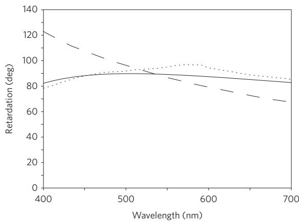
**Figure 4 | Comparative retardation between two man-made quarter-wave retarders and the R8 cell.** Both a quartz zero-order retarder (dashed line) and a subwavelength optimized grating<sup>25</sup> (dotted line) are significantly outperformed by the *Odontodactylus scyllarus* R8 cell mechanism (solid line).
